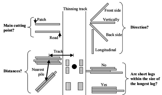
**Figure 1.** Some measured pile characteristics
