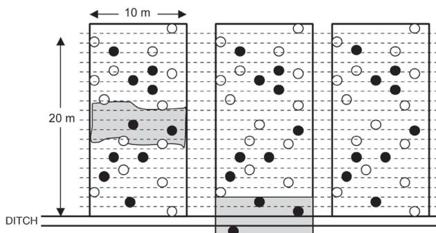
**Figure 1.** Alternative marking methods 1, 2 and 3. Strip roads located in the stand (on the left, Marking 1), strip road located on ditches (in the middle, Marking 2) and no strip roads (on the right, Marking 3)
