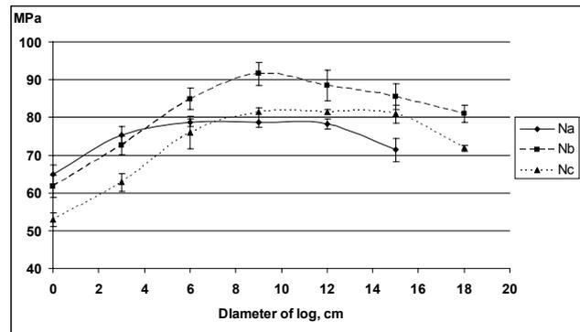
Figure 3. The variation of pine wood compression strength parallel to grain in stem radial direction
