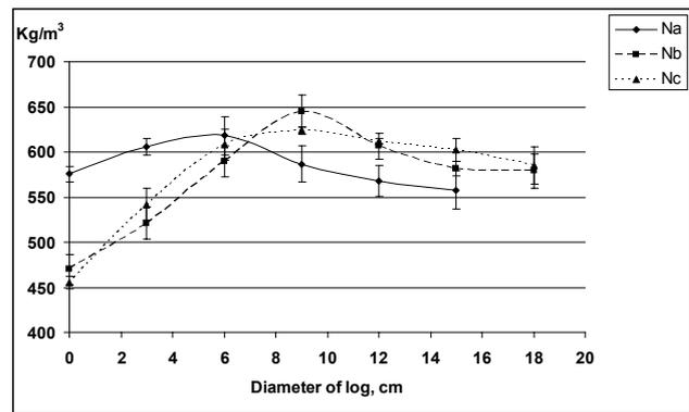
Figure 1. The variation of pine wood density in stem radial direction
