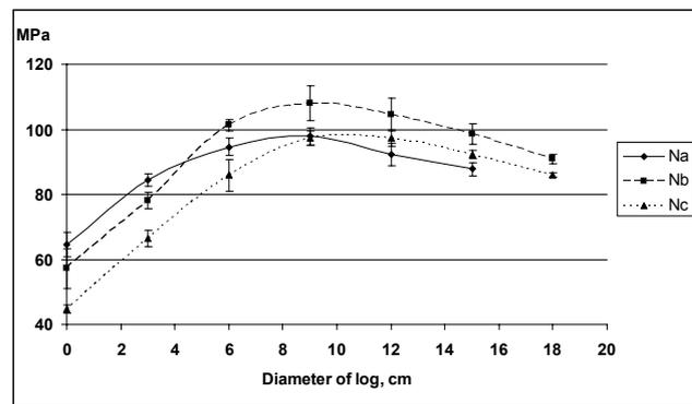
Figure 2. The variation of pine wood bending strength in stem radial direction
