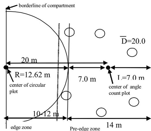
**Figure 2.** Scheme of the edge and pre-edge zone representation by NFI permanent and angle count plots
