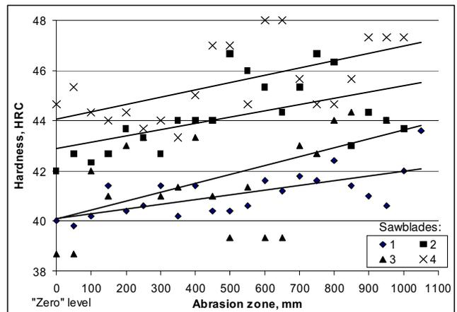
Figure 6. Change of surface hardness within abrasion zone of four tested saw blades
