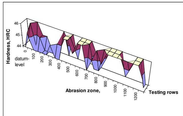
Figure 2. Typical pattern of surface hardness on new frame saw side plane
