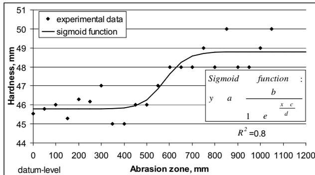
Figure 5. Change of frame saw blade side plane hardness upwards to the top end (sigmoid function coefficients:  $a=45.7765$ ;  $b=3.0248$ ;  $c=578.9751$ ;  $d=47.5412$ )
