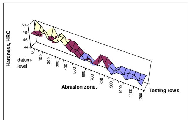
Figure 3. Typical pattern of surface hardness on used frame saw side plane
