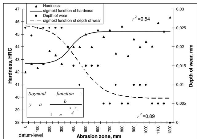
Figure 7. Interrelations of hardness-wear on saw blade side plates within abrasion zone (hardness sigmoid function coefficients:  $a=42.6530$ ;  $b=2.5587$ ;  $c=372.5658$ ;  $d=55.2834$ ; depth of wear sigmoid function coefficients:  $a=0.00643$ ;  $b=0.0194$ ;  $c=438.6372$ ;  $d=-106.8771$ )
