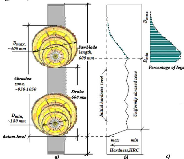
**Figure 1.** Modelling of saw blade abrasion in the kerf within logs contact zone during one frame stroke: a)-location of logs  $D_{min}$ - $D_{max}$  at the upper and lower dead-points of the saw blade stroke; b)-uniformly abraded zone; c)-typical sawlog size distribution
