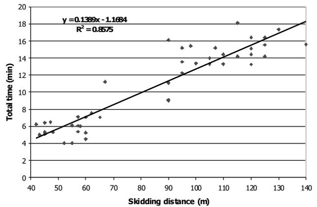
Figure 3. Relationship of skidding distance vs. total time
