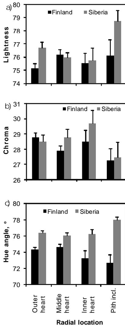
Figure 2. a) Lightness, b) chroma, and c) hue angle of the inner wood of the Finnish and Siberian planks according to radial location
