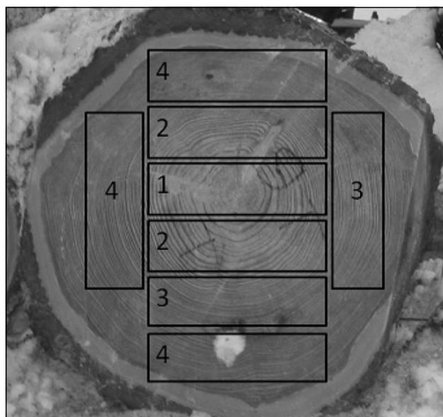
**Figure 1.** Sawing pattern, X-log, used in this study. Numbers refer to the grading of planks according to their radial location in the trunk. The scale used was 1) planks containing the pith, 2) planks from the innermost heartwood, 3) planks from the middle of the heartwood, and 4) planks containing both heartwood and sapwood, referred in text as outer heartwood, because the reflectance spectra were always measured from the heartwood
