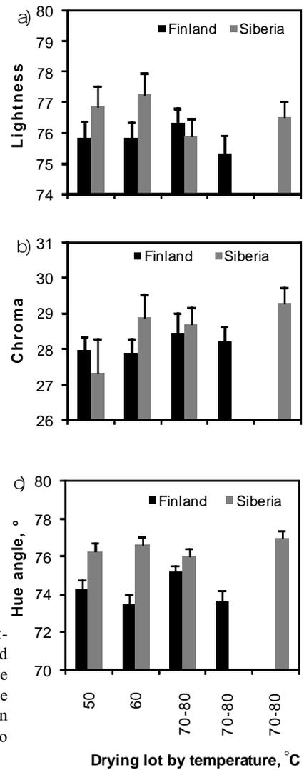
Figure 3. a) Lightness, b) chroma, and c) hue angle of the inner wood of the Finnish and Siberian planks according to drying lot
