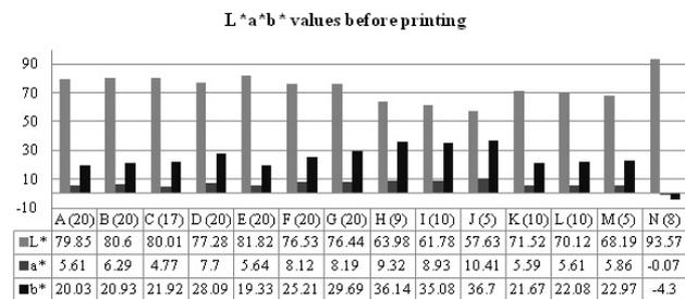
Figure 6. L\*a\*b\* values of the samples before printing, the number of measured samples is presented in parenthesis
