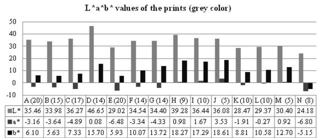
Figure 8. L\*a\*b\* values of the grey printed area on the samples, the number of measured samples is presented in parenthesis. Each sample was measured five times
