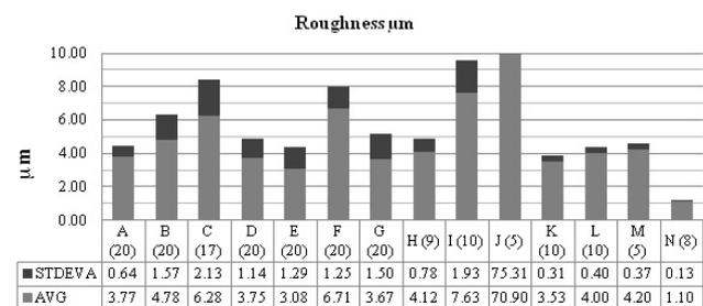
Figure 4. Roughness of the samples (μm), the number of measured samples is presented in parenthesis. The range was set to 160 μm, which was at the highest limits of the machine. In measuring sample batch J, the measuring result went over the limits in 6 measurements of the total 15. These results were marked with the result of 160 μm
