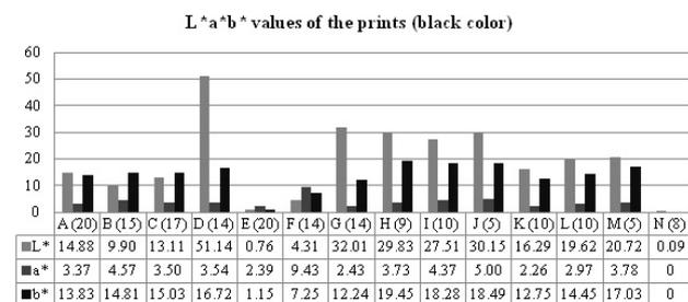
Figure 7. L\*a\*b\* values of the black printed area on the samples, the number of measured samples is presented in parenthesis
