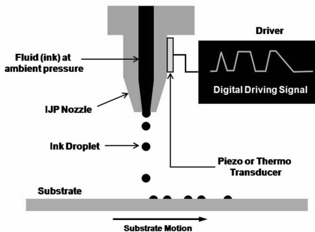
Figure 1. Principle of DOD inkjet printing (SPIE 2009)
