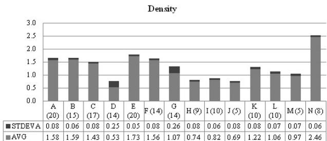
Figure 10. Density of the ink on prints, the number of measured samples is presented in parenthesis
