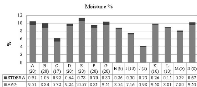
Figure 3. Moisture percentage of the samples before printing, the number of measured samples is presented in parenthesis
