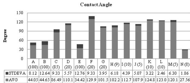
Figure 5. Contact angle of the samples (A, B, C, and E after five seconds of the drop release), the number of measured drops is presented in parenthesis
