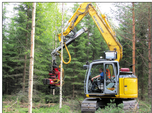
Figure 1. New Holland Kobelco E 135 B SR LC D excavator equipped with Kesla Xtender 15H extension boom and Naarva EF 28 accumulating harvester head
