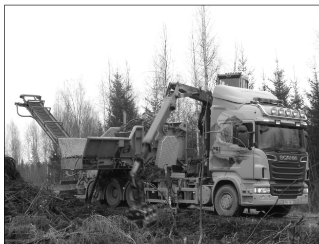
Figure 1. CBI 5800 grinder using a Scania R620 truck as a base machine (Photo J. Laitila, Metla)
