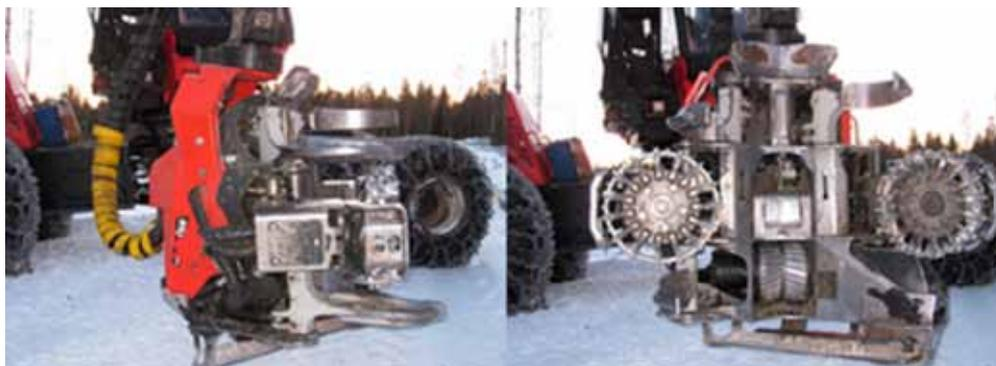
of feed rollers was three, the maximum feeding speed was 5 m/s and cutting was performed with a chainsaw (Komatsu Forest AB).
