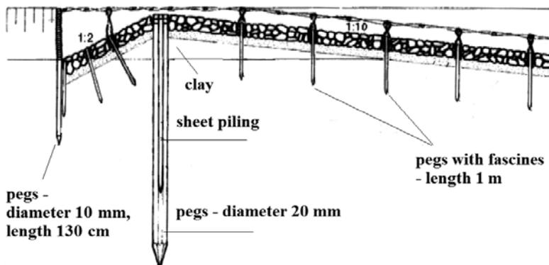
Figure 1. The design of the weir
