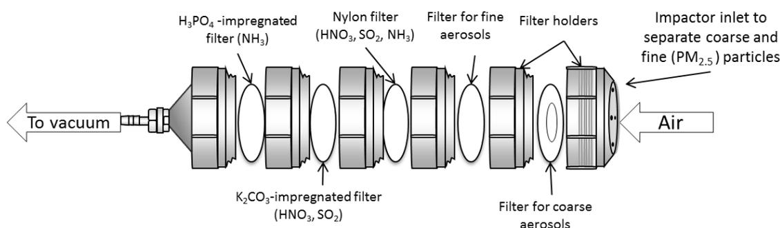
**Figure 2.** Schematic diagram of a filter pack used in this study
