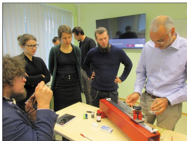
**Photo 2.** Dr. Alan Crivellaro is demonstrating sample preparation using the sledge microtome (photo by Alar Läänelaid)
