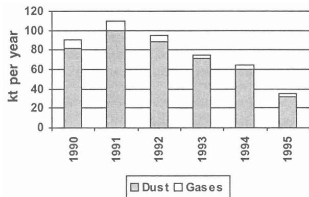
Fig. 2. Emission of dust and gaseous pollutants into the atmosphere from the cement plant in Kunda in 1990-95
